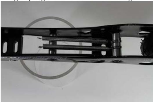
Image: bottom view of frame - axle incl. springs positioned under the rear mounting block
