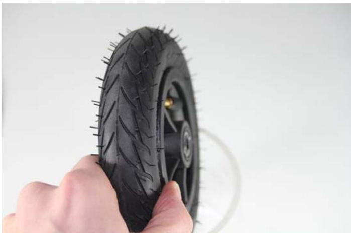
Valve in incorrect position „against“ the running direction
