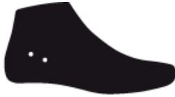
The last is kind of a copy of a foot. The last can have very different shapes depending on the purpose (for example running shoe or speed boot) and target group. The last is important for the fit and performance of the shoe and can make a huge difference.
