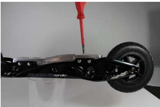
3. fix cone on the clap braket with philipps head screwdriver
