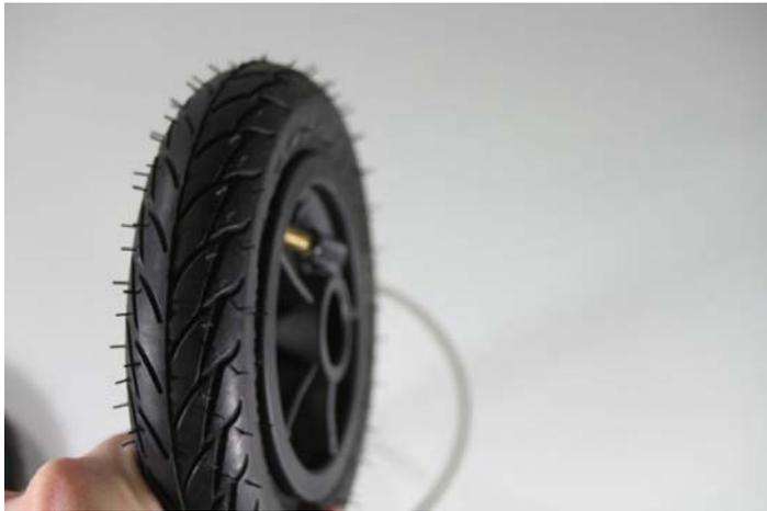
Valve in correct position „in“ the running direction
