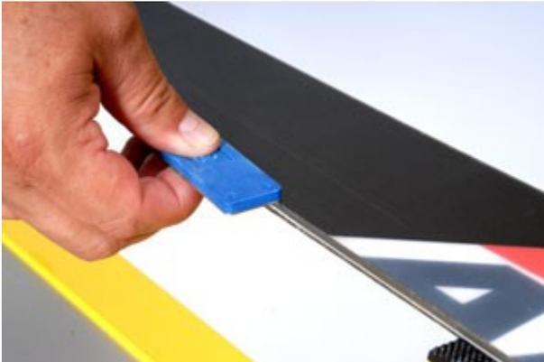
Remove ridges and areas of hardness (caused by stones) with diamond file blue or Universal Edge Grinder.
